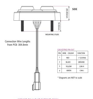
MOUNT ON A FLAT SURFACE ONLY GEC-PKU2200M Part Number: 10-32 UNF S/S Nut Size\*: M5 Spring Washer S/S, M5 Flat Washer S/S Washer Sizes:
